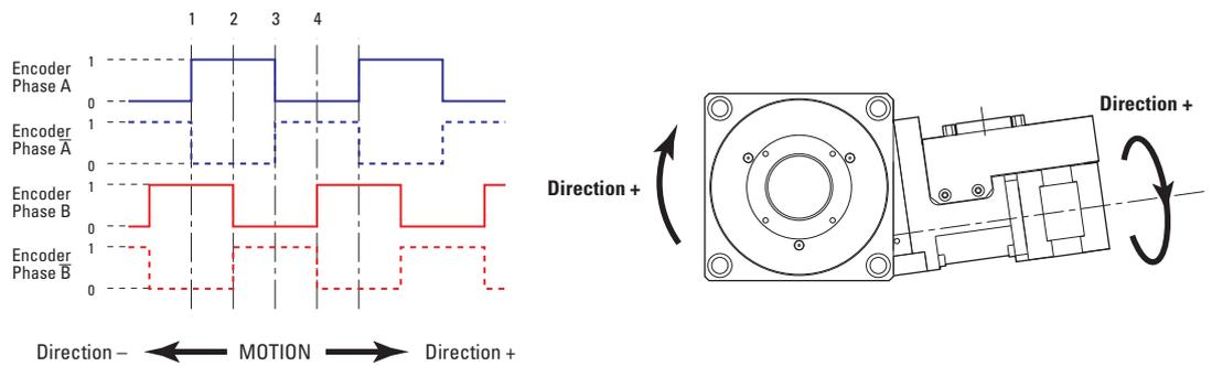
The incremental sensor consists of an optical scale and an encoder head. When the carriage moves, the encoder head generates square signals in quadrature and sends to pins #6, #7, #13 and #14 of the SUB-D15 connector.
