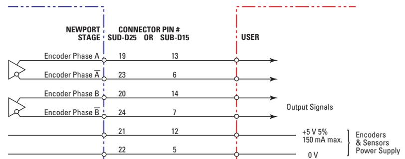
“Encoder” are “differential pair” (type RS-422) type output signals. Using these signals permits a high immunity to noise. Emission circuits generally used by Newport are 26LS31 or MC3487. Reception circuits to use are 26LS32 or MC3486.
