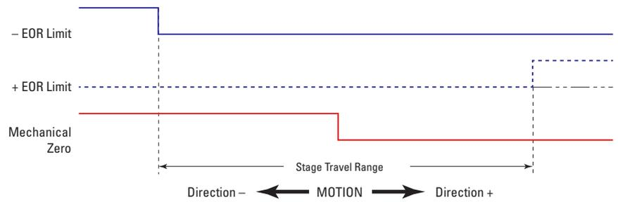
End-of-Run and Mechanical Zero are 5 V open collector type.
